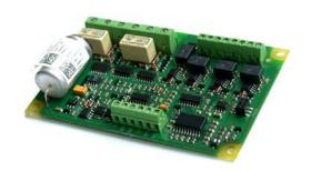
The relay outputs can be switched to a fail-safe position in the event of the X-LINE losing power. This behaviour can be configured and is determined using PC software. The relay outputs are suitable for emitting pulses.
